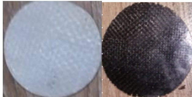
Figure. 2a&2b. Glass fiber and Basalt fiber Epoxy Laminate.
